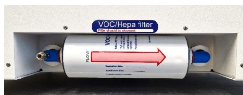
Figura 12.3 Filtru COV/HEPA corect instalat
